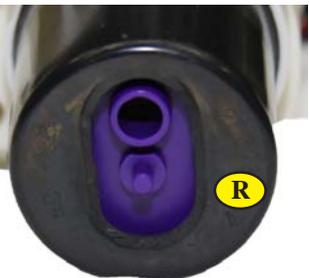
19. Place the Racetronix pump assembly into the fuel module as shown in figures 'S1/S2'. The pump sleeve is keyed in 3 locations on the top so it will only fit in one way.
