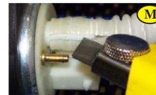
14. Remove the factory fuel pump with its sleeve by sliding it up and out of the fuel module as shown in figure 'N'.
