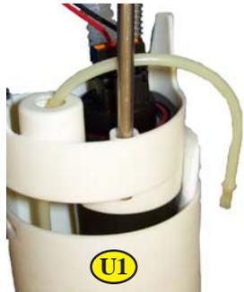
22. Push the venturi tube onto the pump's venturi outlet as shown in figure 'V'. Be careful not to exert excessive side force on the fitting. **Make sure the tube is fully seated on the fitting.**
