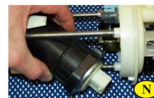
15. Remove the factory fuel pump from its sleeve by pushing out from the bottom. If your pump is older the sleeve will have shrunk from gas immersion. **Do not force the pump out.** If you have the **slightest** difficulty removing the pump from its sleeve simply make a slit down the side of the sleeve as shown in figure 'O'.
